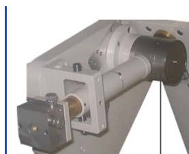
X-Ray optic Germanium or Graphite monochromator
