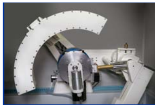
Special thin film attachment θ/Z motorized
